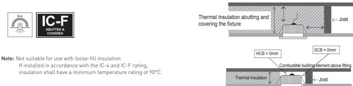
No clearance is required from structural members and building elements (SCB & HCB = 0 mm).
